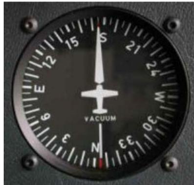
*"Google Images", Sea Gull, Heading Indicator. Retrieved 23 April 2007, from [www.sgsim.com/instruments/DSCN7513-gyro-200.jpg](http://www.sgsim.com/instruments/DSCN7513-gyro-200.jpg)*
