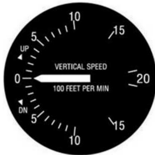
Figure 17B-3 Vertical Speed Indicator Parts
